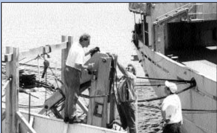
Glacier's fore deck crane needs repair. Keith Holmes, Tom Ebnet and Christian Koether remove frozen hydraulic cylinders in July 2002. It will be returned in January, rebuilt by volunteers ashore. The crane will be operational soon!
