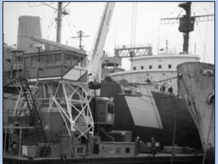
MARAD crane barge lifts pallets and skid boxes of gear to the December volunteer team. Two heavy blava assemblies can be seen moving to the G's bow.
